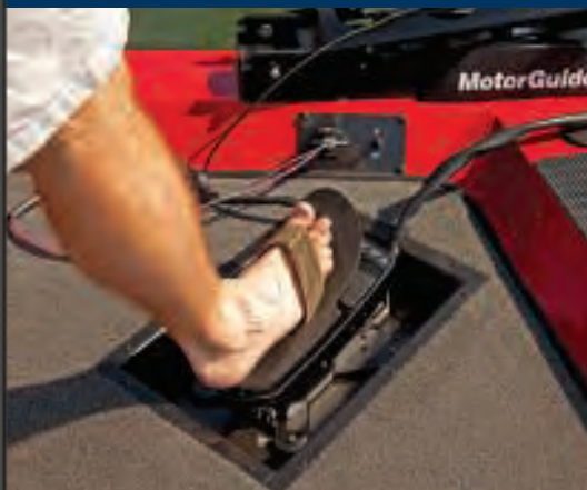
Recessed trolling motor foot pedal (standard)
